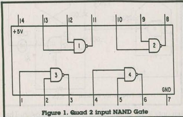
Figure 1. Quad 2 input NAND Gate
