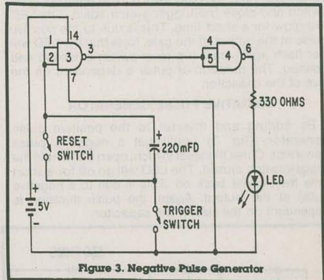
Figure 3. Negative Pulse Generator
