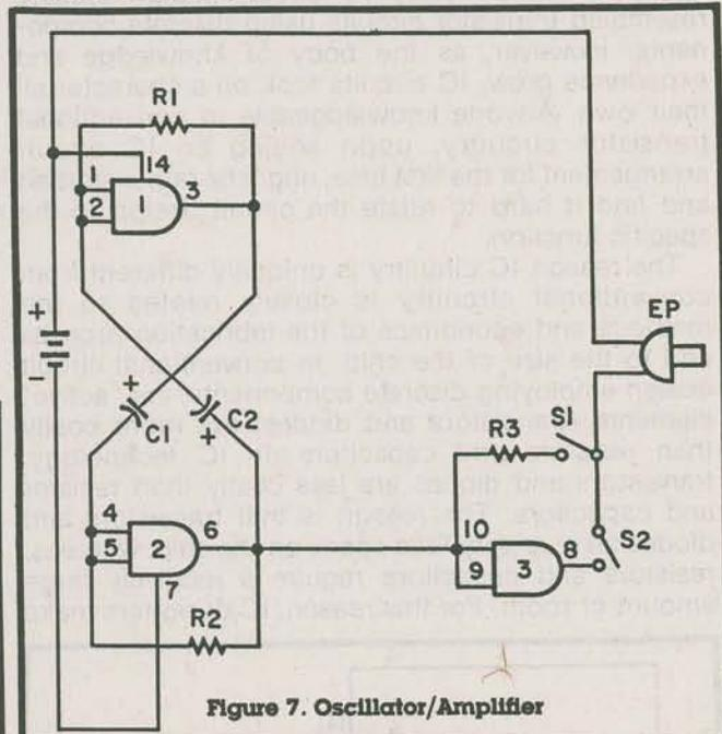
Figure 7. Oscillator/Amplifier
